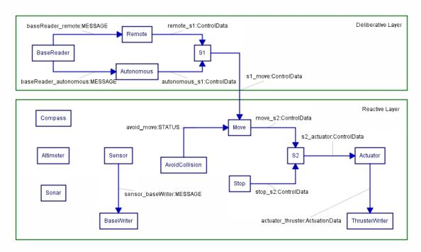
Fig. 3. The LAURS control architecture: processes and channels.
